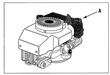
Figure 19: Fill fuel tank.
